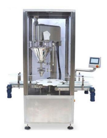
Rotary Automatic Auger Filler with container indexing star wheel and inline checkweigher and rejector, a modular design which allows for filling of different powder products and containers.
