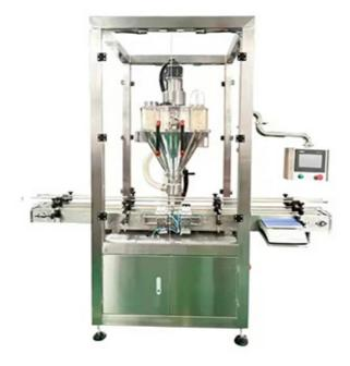
Automatic Single Auger Filler Powder Packing Machine is our new standard type packing equipment for powdery material or fine granules cans/bottles auto packing. This machine is composed of auger filler, S.S304 outside structure, Chain conveyor, Cans seamer&capper etc.
