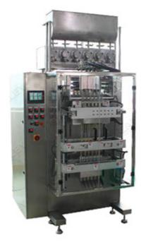
Honey sachet packaging machine can pack liquid or sauce into sachets like water, juice, coconut oil, ketchup, ice popsicle, mouthwash, jam etc. It can be designed with 4 lanes, 6 lanes, 8 lanes, 10 lanes, 12 lanes, etc. The operation of the machine is controlled via a computerized operator interface of touch screen. PLC is programmer for storing many system data.
