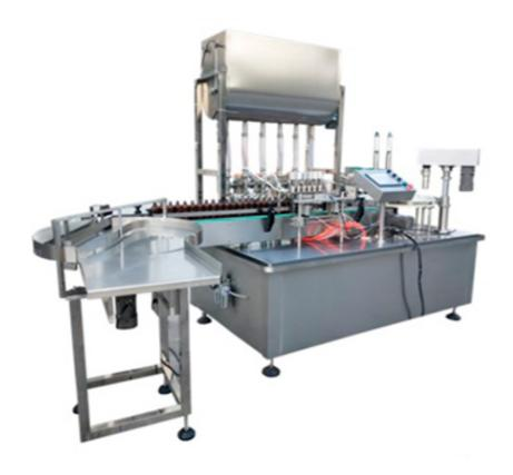
Jam and paste filling is used for filling semi-liquid products without or with small particles: like honey, butter, olive oil, tomato sauce, shampoo, body wish, liquid detergent, etc. The specifications of Jam and paste filling can be customized according to your needs.
