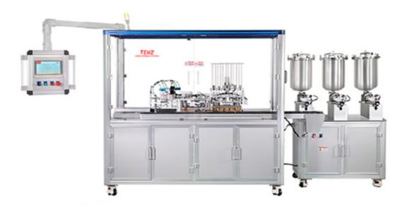
The machine is with 6pcs, push-pull circulation, electric heat sealing, piston type quantitative filling. The main frame is aluminum alloy + 304 stainless steel. The nylon mold is custom made. The machine has a total of 10 molds (The number as per output requirements) cyclic operation.
