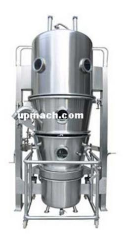
Fluid bed granulator is mainly used for making particles, mixing powder, and drying processes in pharmaceutical, food, feed, and chemical industry. The particles are used as instant drink granules and for filling capsules or compressing tablets.
