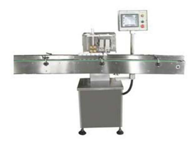
CJ200 cotton inserter is economical and easy to operate. This machine can automatically cut off the belted cotton and insert it into the container accurately and speedily. CJ200 cotton inserter inserts a predetermined length of cotton, rayon or polyester coil into containers at speed up to 70 bottles per minute.
