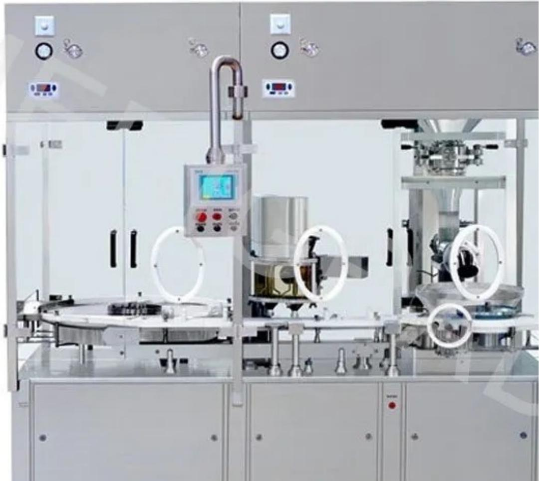
The servo motor is used to control the number of driving coils of the screw powder feeding, so as to accurately control the raw material powder to be packed into the vial according to the specified capacity, and the rubber stopper is covered.
