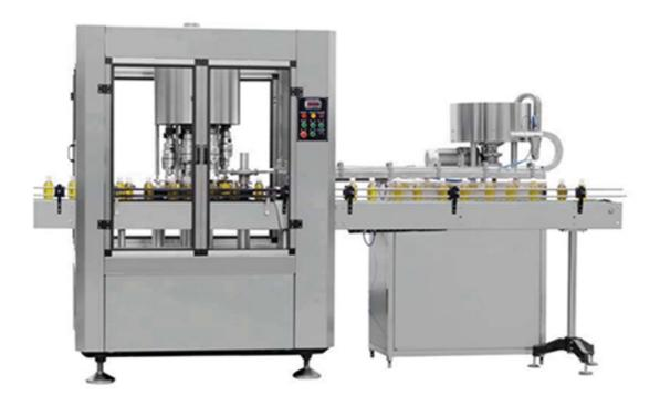
ALC Automatic chuck capping machine for the application of plastic/glass bottles capping. The machine is composed by a conveyor, bottle index wheel, cap unscrambler, cap chute &placer, screwing capper. The bottle loading/unloading through conveyor manually, or automatic directly from an production line. It is designed and made accordance to GMP regulation.
