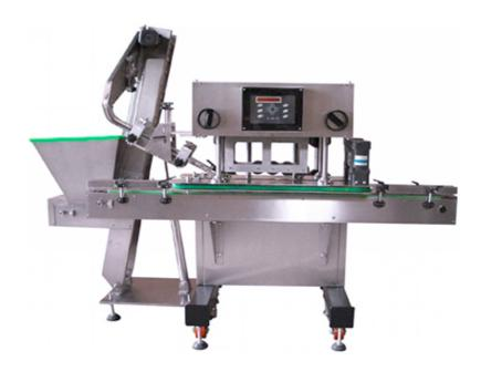
GX200 is economical, and easy to operate. This versatile in-line capper handles a wide range of containers at speed to 200 bottles/min and offers a quick and easy change over routine that maximizes production flexibility.
