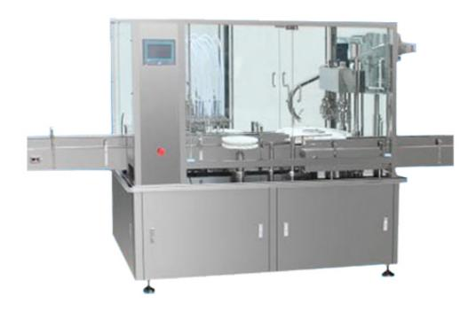
KGT-2 filling and capping machine is suitable for liquid filling and capping in pharmaceutical, healthcare and food industry. The machine design is reasonable, to use single rail to feed bottle, the bottle is transferred by conveying belt, uses 4 piston pump to measure and fill liquid, servomotor and piston pump has been adopted, it has accurate filling volume. It is especially suitable for 30-500ml bottle filling and capping.
