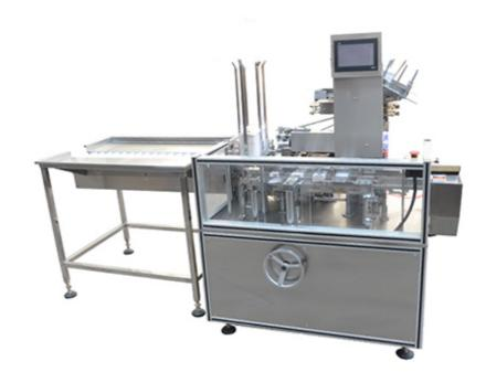
This type is used for ointment medicine bottle (aluminum bottles or plastic bottles). Fold, shaping up and opening automatically of boxes can finished sequentially and automatically, and the batch number on box end is printed automatically. It has functions such as frequency control, PLC automatically controlling, human-computer interface operation system, showing automatically boxing speed and counting.
