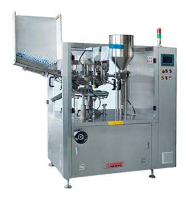
The machine adopts PLC programming controller and full-color industrial touch screen, which can complete the automatic operation of filling ointment cream, gel and viscous fluid, folding (sealing), batch number and other processes. It is an ideal equipment for filling and sealing aluminum tubes, lead pipes. Plastic pipes and composite pipes in the cosmetics pharmaceutical, food, adhesive and other industries.
