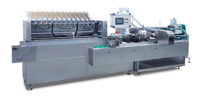
This machine is suitable for sachet, pouch, soft al/al strips, wound plaster, ointment plaster, facial mask plaster, coffee bag into carton. On line product feeding and detecting, leaflet fold (I-4folds) and feeding, leaflet detecting, canton opening and forming, products and leaflet push into carton, printing batch number, sealing carton with tuck-in or hot melt glue device. Automatically reject lacking of leaflet or product and finished product out.
