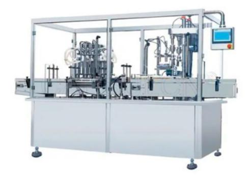
Each CGS-8 Piston Bottle Filling system is specifically constructed to the individual product specifications, space constraints, and production environment to maximize product output. It is an easy to use system with a simple and intuitive touch screen display.
