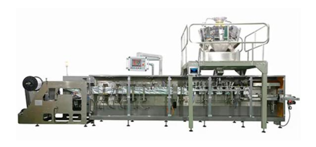
BHD-240SZ is specially designed for doypack bags with zippers. The bag size and filling volume are increased while the accuracy remains unchanged. The maximum capacity of the bag is 2000ml. It is often used to pack large bags of condiments, pet food, chocolate and other powders or granules. In addition to adding zipper function, you can also add hanging holes and other functions according to customer needs, which has a wider scope of application.
