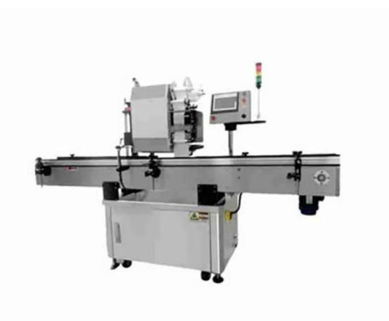
The device is suitable for instant printing and labeling of various label contents. It can realize printing barcode, two-dimensional code, production batch number, etc.
