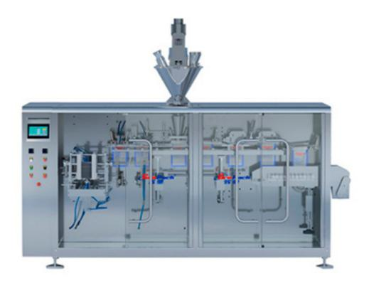
The machine is an automatic packing machine for premade bags. It can meet the requirements which need different specifications, big or small volume but small capacity. It can not only pack 3-side or 4-side sealed bags, but even also bags with hanging holes, standing pouches and shaped bags, and daypack bags with corner spouts, etc. It is applicable to powder, granules, liquid, paste and blocks, etc by using different measuring devices. It is convenient to switch the packing type.
