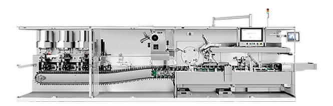
HC 400 is a horizontal carton packaging machine in a continuous motion, in which is capable of producing up to 400 cartons per minute. This model reaches the optimum production while applicable to variety types of products. By incorporating an industry standard PC control system with touch screen, machine operation and production can be easily managed.
