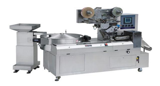
The UN-1200ZS series flow pack packaging equipment is engineered for efficient packaging of multiple small products, such as candies, into a single package. This horizontal flow wrapper utilizes an up-film packing (HFFS) design and is equipped with a vibrating bowl feeder, making it ideal for consistently shaped items.
