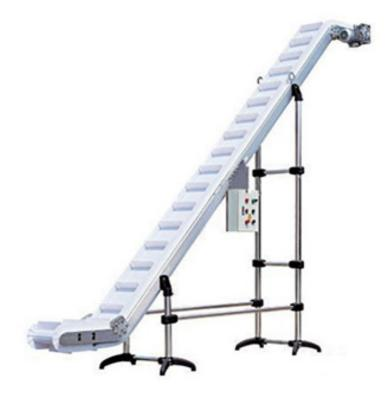
It is adopting modular vent cleat which is suitable for elevating wet products, such as vegetables, fruits, IQF frozen products, the water will drip on the bottom collecting plate. Certainly, it's also used for other dry snacks, candies, cookies etc products' delivery. Its height is available to be customized design as the clients' requests.
