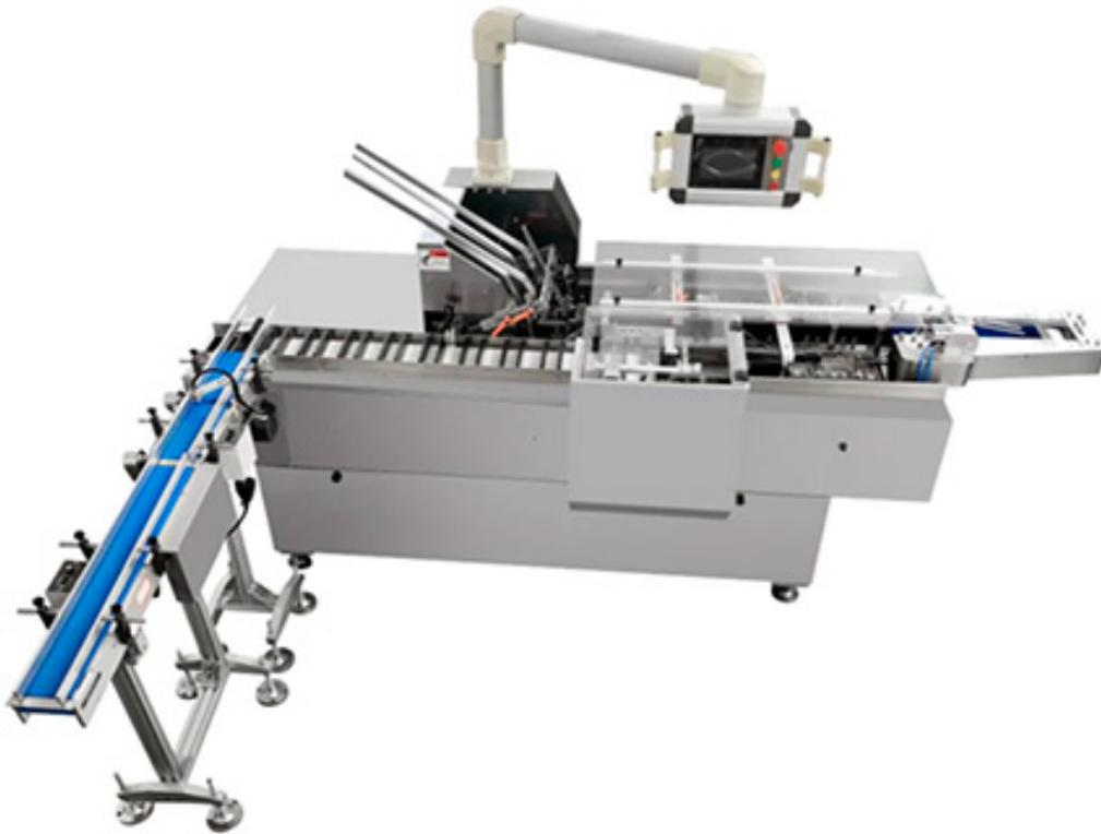
The Automatic Horizontal Cartoning Machine is a highly versatile, high-speed packaging system designed for packaging various items, including blister packs, bottles, tubes, soap, and other items in the pharmaceutical, food, cosmetic, and daily chemical industries. It employs a chain-driven, unidirectional transmission system for smooth, stable operation and a broad adjustment range, making it suitable for a wide range of products and packaging requirements.
