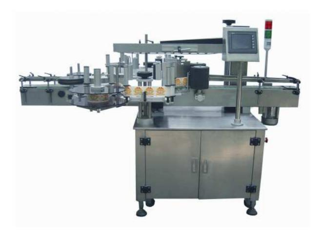
This machine is applied to label the self-adhesive label on various cylindrical bottles, flat bottles, and Square bottles. Suitable for double side and single side labeling.
