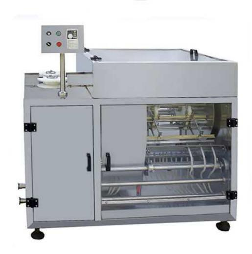
Applied for all kinds of material or irregular bottle from 30ml to 500ml which have bolder, the machine can wash the bottle inside and outside. Adopt two times of water and one time of air to washing bottle (drinking water-WFI-purified compressed air), and washed bottle comply with requirement and dry.
