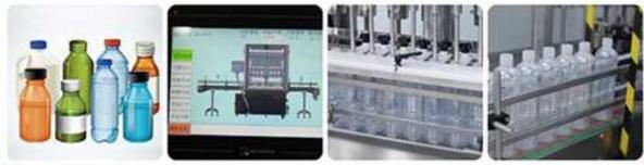
An inline filling machine specially designed to meet the need of the demanding users. Suitable for filling liquids of different viscosity like medicines, syrups, oil, and cream etc. Independently and electronically controlled filling nozzles offers high precision, easy setup and adjustment, as well as high versatility. Capable of mixed filling requirements within the group of nozzles. Pre-set product program allows fast changeover.
