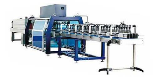
Self-supporting frame with sliding doors which makes machine control and maintenance easier.
