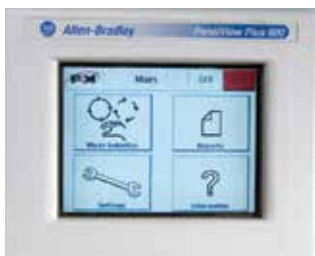
PLC control system with color touch screen graphical interface for easy operation and maintenance
