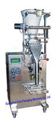
It is wildly used in medicine, foodstuff, the chemical industry of grain, pills, powder, etc. All the works of bag-making, date printing ration filling, sealing-cutting. It is made up of stainless steel and up to International Health standard. The machine is reliable and operates easily, few stoppages. It has a good reputation in home and abroad.
