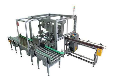
Auto carton filling machine is specially for small boxes loading and filling system. It is automatically accumulating products and auto loading into cartons. It is working stably and high speed widely applied on the chemical products, food and other small boxes, and products loading packing solution.
