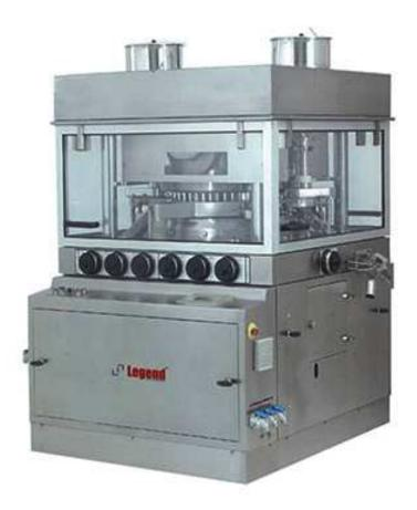
Legend Septa Press Double rotary tablet compression machine (GMP model) with maximum output up to 583, 200\* Tab/Hr. (Max).available in D", B" & BB." tooling. It is an Advanced High Speed Tableting machine enhanced with Hydraulic Power Pack system & Auto Lubrication With Excellent accessibility for quick cleaning. Suitable for large batch production.
