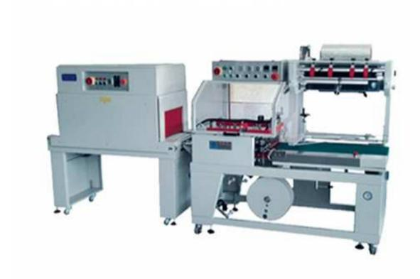
It is used to pack kinds of small components, appliances and objects with POF, PP or PVC film etc, such as electrical products, hardware, software, wallpaper, cosmetics, food, printing products, medications, floor boards, ceramics etc.
