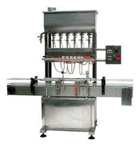
The machine adopts the principles of design time control flow, filling volume, especially suitable for filling liquid products better mobility, the majority of wine, cosmetic, detergent, pharmaceutical and food industries ideal for low viscosity products filling machinery
