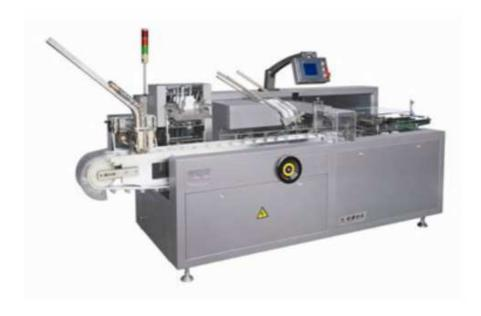
This machine is suitable for cardboard case packaging for blister packing. It consists of direction folding (1-4 folds) and feeding equipment, cardboard case forming and feeding, batch number printing, sealing of case tongues at both ends ect. The whole encasing process is finished automatically. It can be added hot-glue machine.
