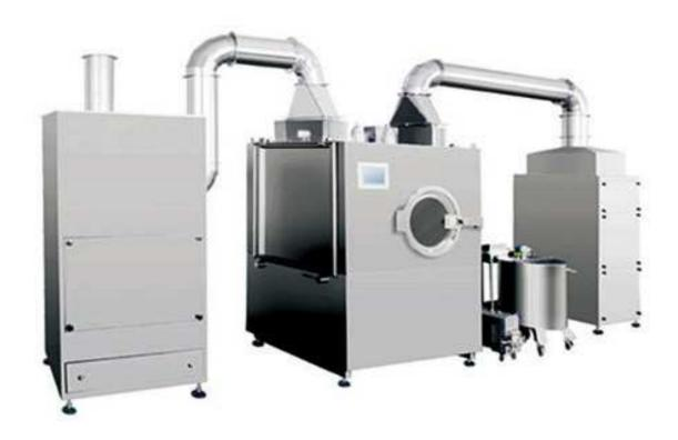
The SED-150GB Film Coating machine is kind of equipment integrating elegance, high efficiency, energy-saving, safety, easy to clean, which is applied for coating traditional Chinese and Western tablets and pills (including micro-pills, small pills, water-bindered pills, drip pills and granulated pills) with sugar, organic film, water soluble film, slow and controlled release film in the fields of pharmacy, food and biology etc.
