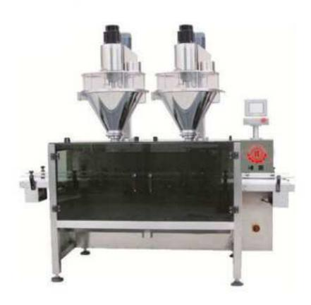
This machine is mainly controlled by mechanical, electrical control, conveyor belt, photoelectric detection, powder filling device, a bottle body, a touch screen. The powder or granule feeder can choose by you. This machine applies for food, pesticides, cosmetics, pharmacy industries of the powder, granule product automatic filling.
