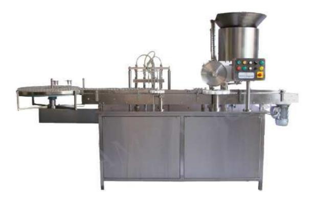
The incoming dry vials (sterilized and siliconised) are fed through the in-feed turn table and suitably guided on the moving delrin slat conveyor belt at the required speed of the correct placement below filling unit. The filling unit consists syringes & nozzles uses for the filling. The vials in a raw are stopped under the filling nozzles by the star wheel rotating indexing mechanism for filling operation and move further to stoppering station for stoppering operation.
