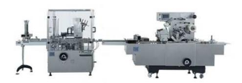
Model DZ-120B Cartoner machine is suitable for packing blister cards. On line product feeding and detecting, leaflet fold (1-4 folds) and feeding, leaflet detecting, canton opening and forming, products and leaflet pushing into carton, printing batch number, sealing carton with tuck-in or hot melt glue device. Automatically reject lacking of leaflet or product and finished product out.
