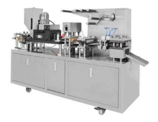
The product is specially designed for hospital dosage room, laboratory institute, health care product, middle-small pharmacy factory, and featured by compact machine body, easy operation, multi-function, stroke adjustable, long durability etc, it is suitable for the Alu-PVC package of medicine, food, electric parts etc. Aided forming Pre-cutting Inspection and rejecting control systems. Print mark registration Automatic feeder
