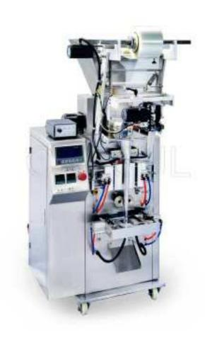
Automatically measuring volume, making bags, filling, sealing, cutting, printing the lot number and cutting easy tearing notches, making chain sachet, finished product conveying.
