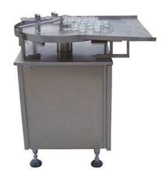
This bottle turntable, also called infeed turntable, is an indispensable auxiliary machine for connection and transmission of automatic filling production line, and it conforms to related GMP standards. Its main component is the turntable device.
