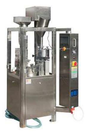
Small fully-auto capsule filling machine NJP-400C processes the products for optimal productivity up to 400 capsules per minutes, featuring low-maintenance operation, minimal downtime, and overall dependable production.
