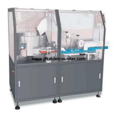
This bottle unscrambler has much faster speed, can be adjusted steplessly, which is convenient for production arrangement. Is used to plastic round square irregular bottles range from 15ml-500ml, equipped with tablet counting or liquid filling. This unscrambler is fully conforming to GMP requirements. It is widely used in the industries such as pharmacy, food, chemical engineering etc.
