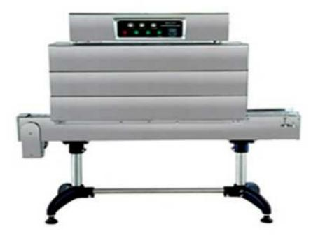
This series label shrink machines are mainly used to shrink label of product in bottle shape, can shape or barrel shape with glass bottle, plastic bottle or paper cup. The label either on the top, in the middle, at bottom of bottle or wrapping the whole bottle is able to be shrank with different type model. It is widely applied in the industry of food, medicine, cosmetic and pesticide, etc.
