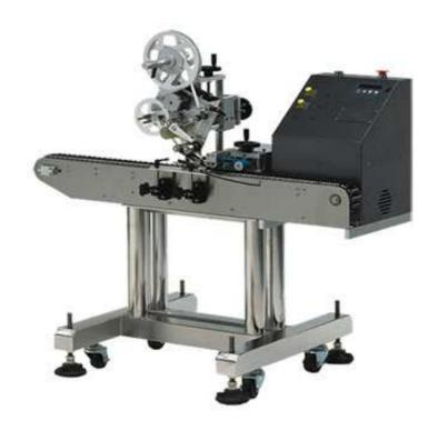
GRL-003 is derived from GRL-002. It is mainly aimed at cylinder which is oversized in length and diameter, unable to stand steadily. This machine will be the best solution, such as Ampule bottle, pen, pen type glue, etc.. Meanwhile, it still can maintain speed above 100 bpm with high accuracy.
