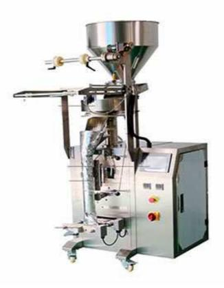
This machine is widely used to pack any loose, non-cohesive granule products of the food, pharmaceutical, and chemical industries, such as soup mix, coffee, instant drink mix, desiccant, monosodium glutamate, sugar, salt, cereal etc.
