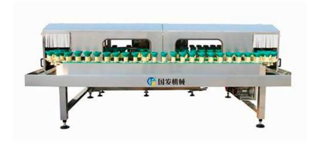
Wear resistant polyformaldehyde molded chain link, using special structural design to make it and the dumpling chain shaft relatively static without sliding friction never wear, overcome the type of punching control machine chain not to use, short life, high cost of the common industry.
