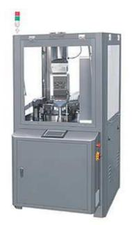
NJY-100C hard capsule filling machine is a device designed and produced by our company. It can be filled in a hard capsule (solution, suspension, micro emulsion). The ceramic pump is used to add liquid, and the servo motor controls the loading system to ensure the difference in loading, accurate measurement, fiber inspection, lack of glue, and automatic kicking.
