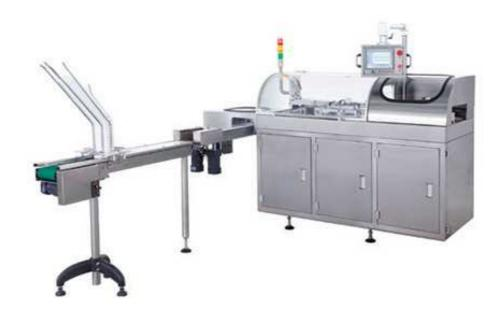
The machine can be used to pack single or multiple medicine box, tobacco, food and with BOPP or PVC film. The max speed is 30 packs /min. It can finish all actions automatically like stuff-stacking, feeding, packing film feeding, folding, packing, heat-sealing and so on. The machine uses mechanical transmission, frequency convert, HMI and PLC to control. The malfunction can be shown automatically when the machine is running. It can be used separately or in line with automatic boxing machine.
