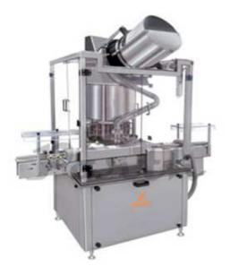
Automatic ROPP Cap Sealing Machine is versatile, self-supported on stainless steel leg with height adjustable adjustment system. This ROPP Capping machine is precision built on sturdy welded MS frame completely enclose in stainless steel sheet and doors are providing to facilitate the servicing of machine.
