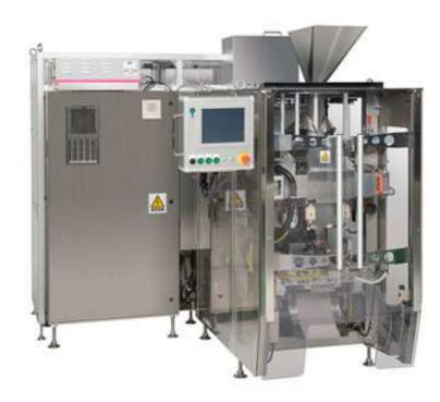
Vertical Form Fill Seal machine(VFFS) forms bag from film and fills an assortment of products such as powders, granules, and pieces, which come in a variety of shapes and kinds of foods such as candies, coffee beans, frozen foods and snacks by dropping vertically.
